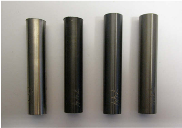
Fig. 1. Five centimeter long tube specimens of Zircaloy-2 (from left to right:) un-oxidized; with 1 \mu\text{m} thick oxide; with 2 \mu\text{m} thick oxide; and with 9 \mu\text{m} thick oxide. (For interpretation of the references to colour in this figure legend, the reader is referred to the web version of this article.)
